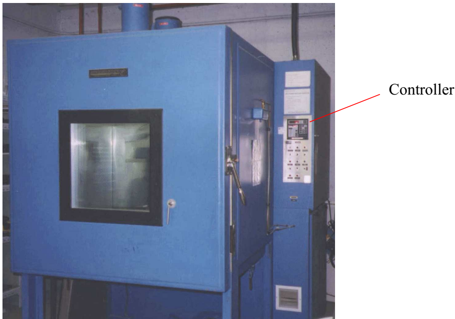
Figure 1: Weir-Jones Engineering Consultants Ltd. environmental chamber.
