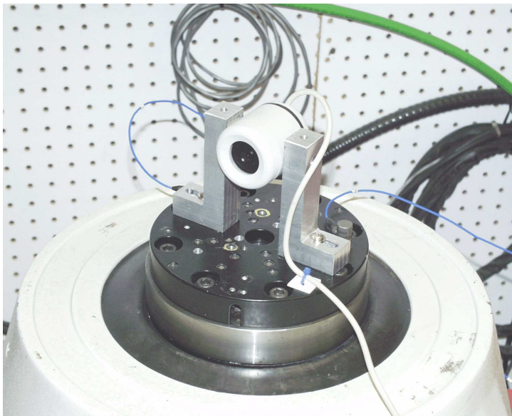
Figure 4B: Transverse orientation mounting of the CCTV camera.
